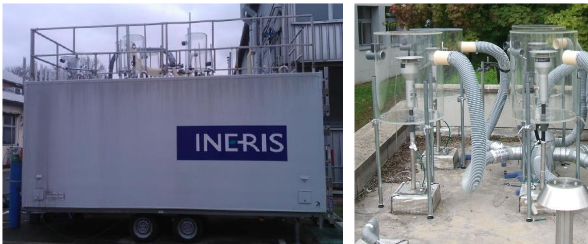
Figure 4: Test trailer (left) and doping cylinder (right) used in inter-laboratory comparison exercises of PM automated analysers.
