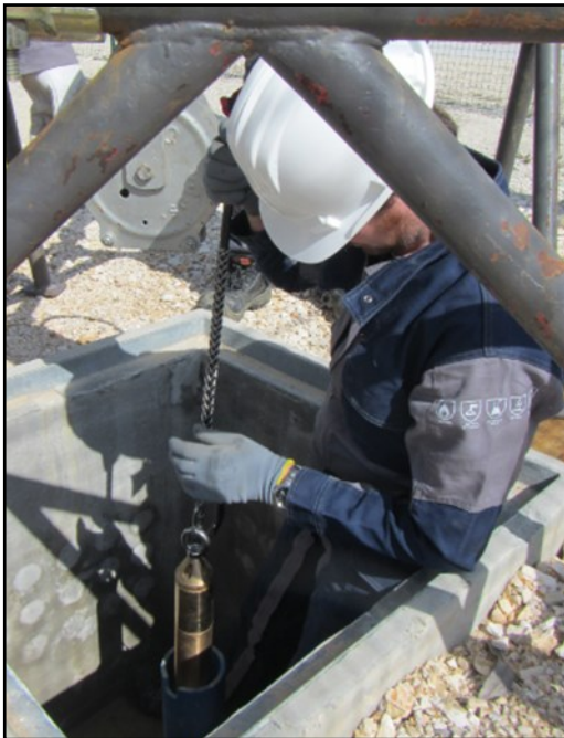
Installation of a downhole SYTMIS 3-component retrievable microseismic probe.
